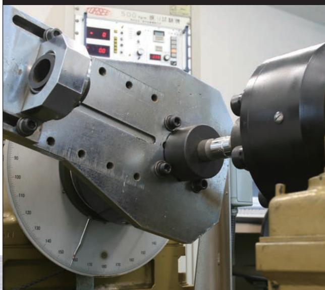
Ko-ken uses a variety of test equipment. Strength is measured by the Static Load Test Machine that can measure torque load up to 5,000Nm. Durability is measured by the Cyclic Test Machine and corrosion resistance testing is done by the Salt Spray Test Machine. The test results are used to improve our standard products and assist with new product design and development.
