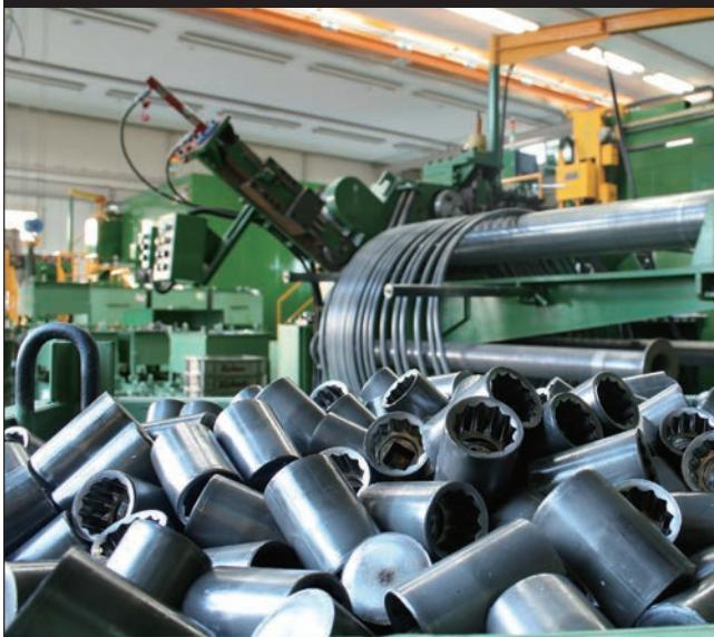
The Forming machines are used for the forging process. These machines can produce mass quantities of sockets and parts with high accuracy that ordinary drop forging machines can not achieve. On the other hand, ordinary forging machines are also used for small production runs.
