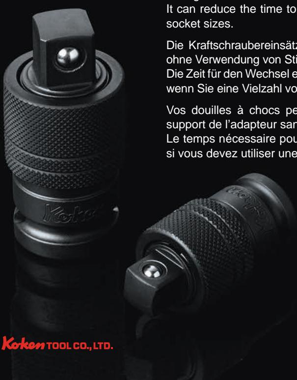
Impact sockets can be attached or detached on the LOCKING ADAPTOR for safety just by sliding the holder rather than using a pin and an O-ring.
