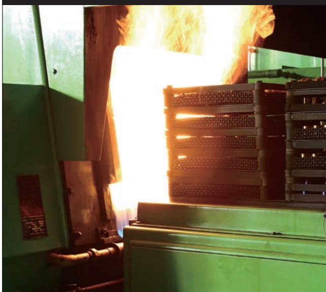
To make the tools stronger and more durable, proper heat treatment is critically important. The temperature and the time of the heat treatment are strictly regulated by a very accurate control device.
