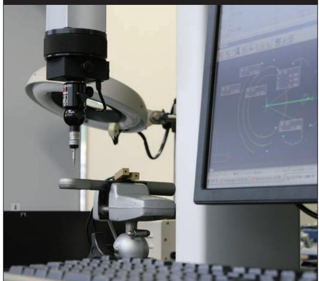
Our products are periodically checked at each production process by inspection devices. Highly accurate 3-D measuring instruments are used to inspect and confirm dimensions.
