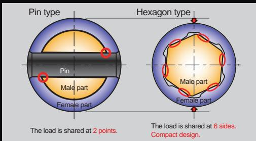
Ball type universal joints use a new structure of joint mechanism without a pin. Being connected by mutually engaged hexahedrons, the load is dispersed across the whole outer circumference.
