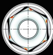
Flat Drive is designed to guarantee a flat surface contact between the socket and the bolt/nut.
