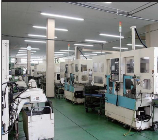
The forged steel is turned into required shapes and dimensions. The MC (Machining Center) operates with extraordinary speed and precision. The article number, size, logo, production number, and MADE IN JAPAN are marked on the products after the turning process has been completed.
